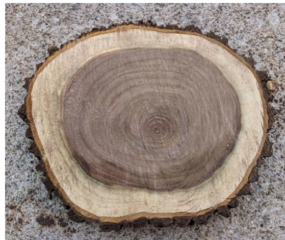
Figure 5 - Walnut tree cookie showing heartwood (brown) and sapwood (white). (Photo credit: Future Generations University)
