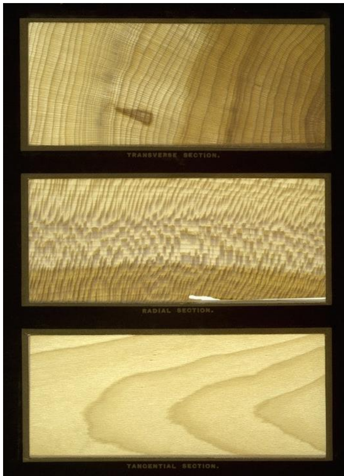
Figure 3 – Photo plates demonstrating different cuts of sycamore lumber. The uppermost image is a transverse cut, demonstrating the growth rings and the color change between heartwood and sapwood. The middle image is radial section cut which demonstrates the visual aesthetic of quartersawn sycamore lumber. The bottom image is a tangential section, demonstrating a plain-sawn board. (Image credit: Romeyn Beck Hough, Hough and Hough 1888)
