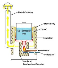
heat to the pan. It was designed as a cook stove for use in developing countries, as a way of reducing deforestation. Although the maximum heat may not be ideal for sautéing vegetables, it is ideal for boiling sap. The syrup was then moved to a propane burner and finally finished off on a kitchen stove.
